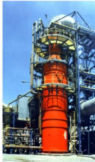
Figure 1. Schematic representation of a venturi scrubber.
